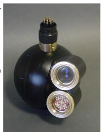
Weighing in at only 3.6 Kg and able to fit through a 185mm diameter hole, it can be deployed in situations that exclude other cameras.
