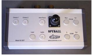
Model SCDDT-I has push button controls for operation of two Model SBCI Inspection Spyballs. (Any other Spyball version is also compatible although some controls would not be required)
