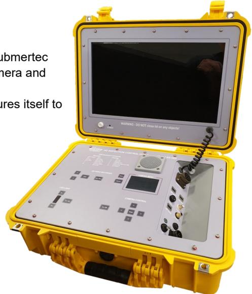
The built in Digital Video Recorder (DVR) stores 1080p MP4 video and 1920x1080 JPG photos to internal 256GB memory with simultaneous recording to removable USB Memory if required.
